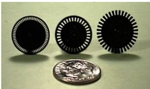
Left - Apple USB Mouse: 65 spokes Middle - Umax SuperMac Mouse: 34 spokes Right - Kensington USB ValuMouse: 36 spokes
