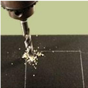
Drill a hole inside the rectangle you just marked using the 3/8" drill bit. The hole has to be big enough to fit your jigsaw blade into.
