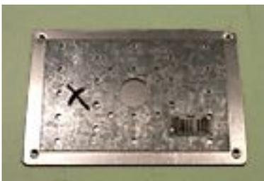
Line up the steel plate used for the spinner assembly on the aluminum lid that came with the project box. Center it as closely as possible.
