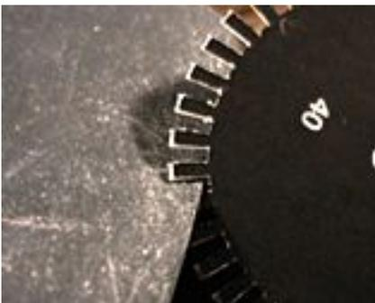
Use fine grit sandpaper to clean off any rough edges where plastic or the paper didn't cut off cleanly.
