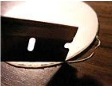
After the adhesive sets up, use a razor to trim any excess paper from the edge of the disc.
