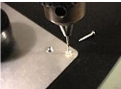
Use the 1/16" drill bit to make pilot holes in the wood at all four corners. Work the drill up and down to clear out the holes.
