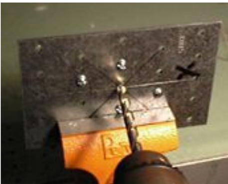
Clamp the two plates into a vice, and drill out the center hole with a 1/4" bit.
