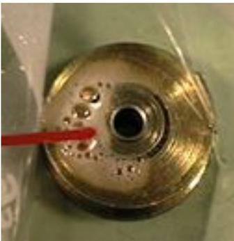
Take the roller, and blast WD-40 into the channel where the ball bearings are. The idea here is to remove all of the heavy grease that's packed in there. This may take a bit of time to do. Periodically wipe away the grease with paper towel as you work, and spray from both sides. You'll know you're finished when the bearing spins freely. I put the roller into a plastic bag to do this, so I didn't get WD-40 everywhere.
