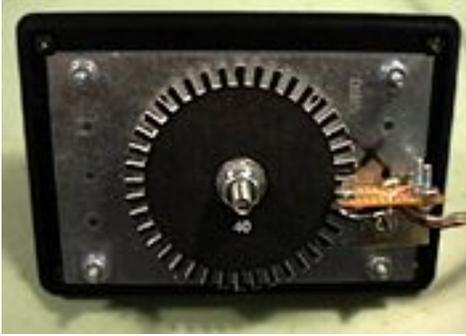
Reattach the shaft and encoder wheel, and realign the bracket. Everything goes back together the way it was assembled the first time.
