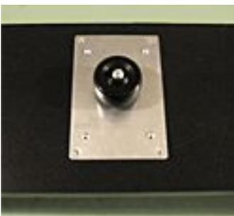
Attach the spinner to the control panel using the screws that came with the project box. Go slowly and don't overtighten the screws, so you don't tear the wood out.
