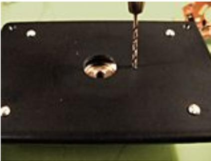
Use the 3/32" drill bit and start the hole by drilling straight down about 3/8" away from the edge of the center hole.
