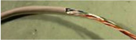
Remove the outer sheath from the wire you're using (scrap category 5 ethernet cable is shown). Cut the wire to about 6" to 8" in length.
