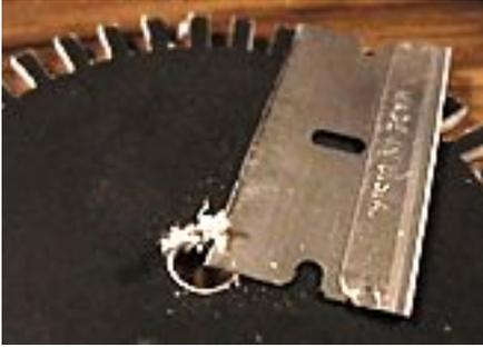
Use the razor blade to trim off any excess paper or plastic from around the edge of the hole.
