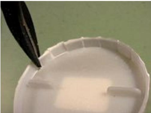
Use tin snips or a fine toothed saw to make cuts all the way around the rim, about 1/4" apart. Then, use the pliers again to break off the pieces.
