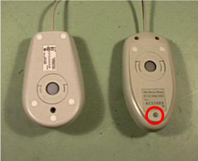
Take your mouse apart. Generally, there will be one or two screws. Sometimes hidden under labels or glides, as shown by the red circle. Once the screws are out, usually you have to pry the back end of the mouse up to pull it apart.
