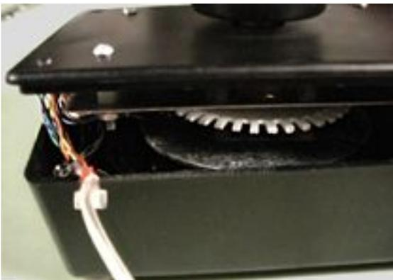
Use the same wire-stuffing method from before to close the lid. You will have to drop the lid almost straight down into the box for the counterweight to fit.
