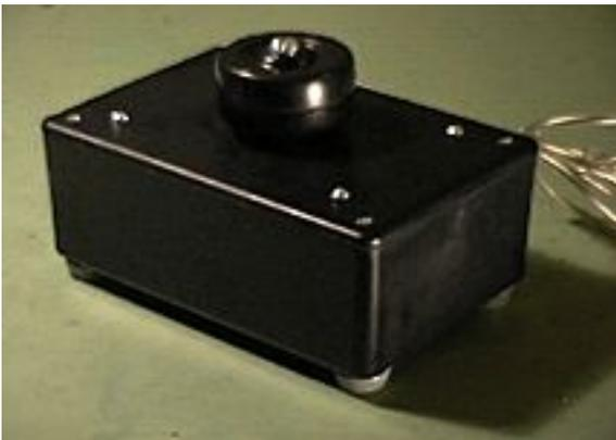
Once the lid is closed, screw it down. You now have a finished spinner! The knob should spin freely. If the knob feels a bit light, you can go back and add a counterweight to it for an even better arcade feel, as shown on the following pages.
