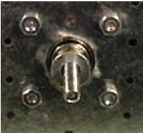
Place a 1/4" washer on the end of the shaft. Try to find the flattest one you can.
