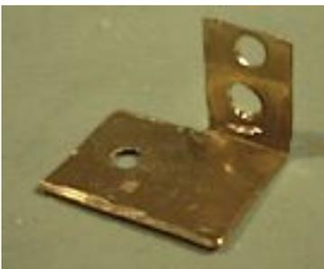
Cut the bracket along the line you scratched into it earlier. File off any rough edges.
