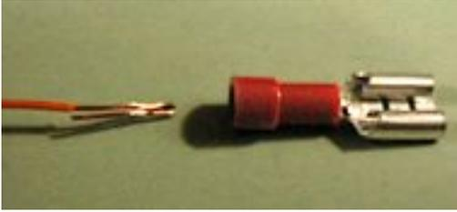
One at a time, cut all **except** the common (brown) wires to length - so they easily reach the terminals on the switches. Strip 1/2" of insulation off of them, and double them over as shown.
