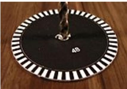
Slowly drill through the plastic with a 1/4" drill bit. Put a piece of scrap wood under the disc for support.
