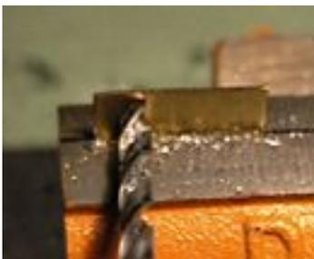
Use a 5/32" drill bit to drill the two holes you marked with the centerpunch. You're using a larger bit so that you'll be able to make adjustments later, if necessary.
