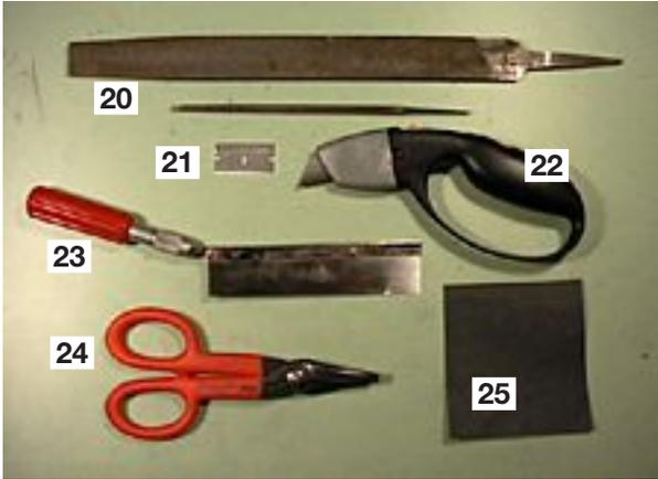
20. **Files.** You should have a flat file, and a small round one. Used for cleaning the rough edges off cuts and holes.
