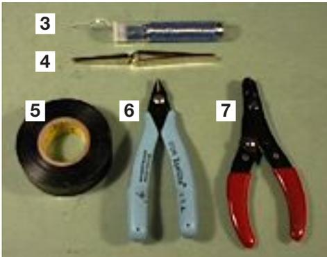
3. You'll need some **rosin-core solder**. Get some that says for it's for fine electronic soldering or circuit boards (63% lead/37% tin). **\$2.99**
