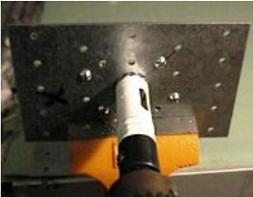
Remove the roller again. Use the 3/4" hole saw to drill out the center hole. Let the saw do the work - don't force it into the metal.
