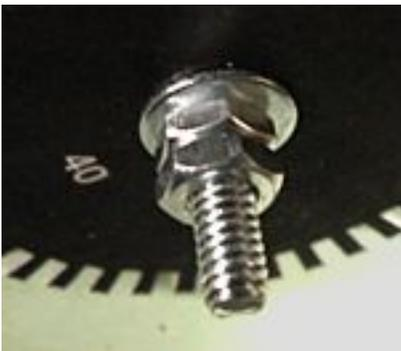
Place two 1/4" jam nuts on the shaft, and tighten them down.
