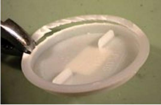
Take the ABS plastic test cap, and use a pair of pliers or an adjustable wrench to remove the edge of the rim. Work a short section back and forth a few times, until it breaks free, and do this all the way around.
