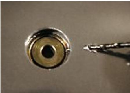
The same procedure applies to the aluminum plate used for control panel mounting. However, with the aluminum plate it's especially important to remove the spinner assembly and clean out any metal shavings, and also file down the rough edges on the bottom side of the aluminum.
