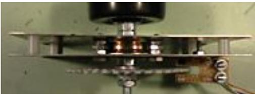
Place the four spacers between the metal plates, at the corner holes (which you used to drill holes in the box lid earlier). If they don't stay in place, use some glue to hold them.
