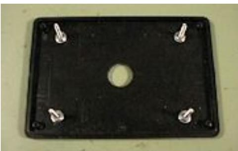
Push four 1" long #6-32 screws down through the holes in the lid of the project box. Attach each one with a #6 washer and nut from the underside.
