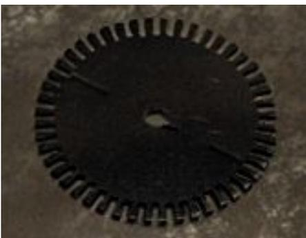
Sand both sides of the disc, so there aren't any bits of plastic sticking up, then give it a couple of coats of flat black spray paint. This may not be completely necessary, but since the disc isn't completely opaque, there's always the chance an errant signal could get through.
