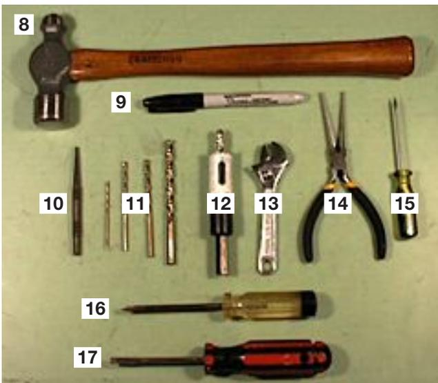
8. **Hammer** (for using the centerpunch, and flattening out unruly pieces of metal)
