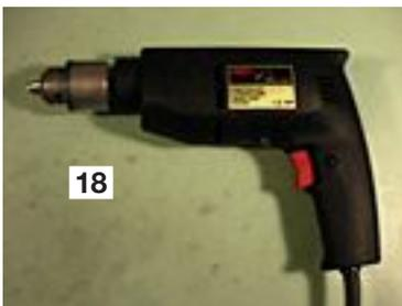
18. **Drill**. Preferably a variable speed, reversible model. You'll be drilling through plastic, steel, brass and brittle circuit board material. It will also need to have a chuck large enough for the hole saw.
