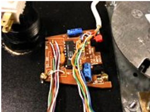
Attach the circuit board to the underside of the panel as described on **page 40**.
