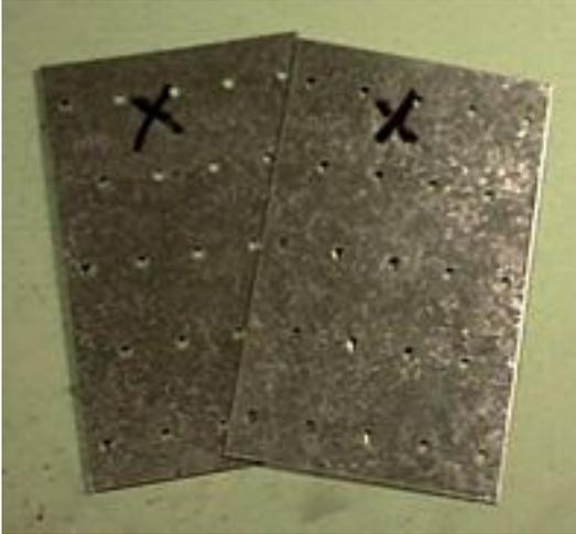
Line up the two metal tie plates so the holes match. Put a mark on each plate so you can keep them oriented.
