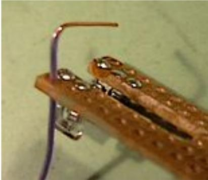
Push one wire through the circuit board from the top side, and bend the bare part of the wire over at 90°.
